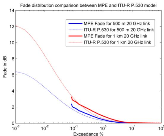
**Figure 7:** Fade distribution comparison between MPE and ITU-R P.530 model for Peninsular Malaysia
