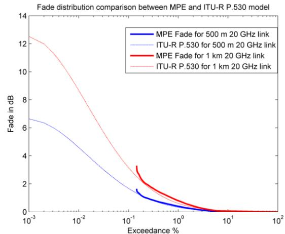
**Figure 8:** Fade distribution comparison between MPE and ITU-R P.530 model for East Malaysia
