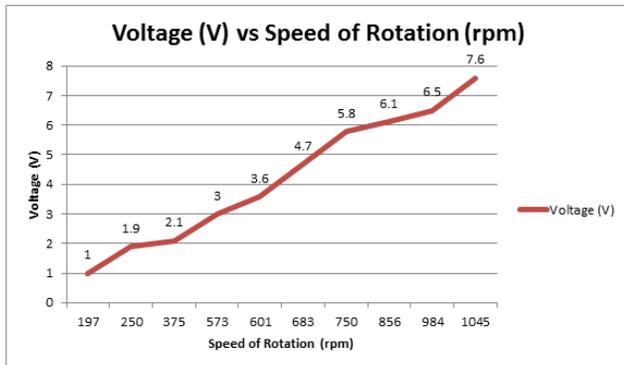
Fig. 6. Graph turbine speed versus AC voltage output
