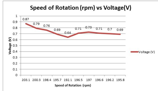
Fig. 4. Graph turbine speed versus AC voltage output
