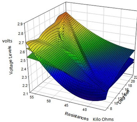
Figure 10: Comparative analysis of voltage levels in terms of both bending and resistances.
