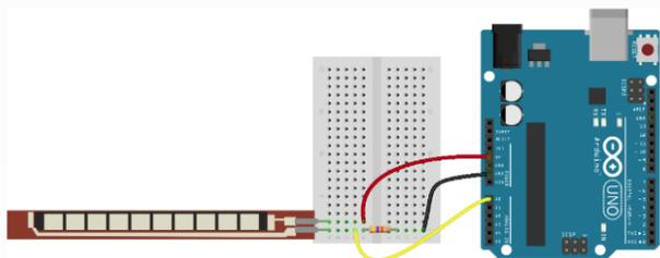
Figure 3: Flex sensor resistor measurement
