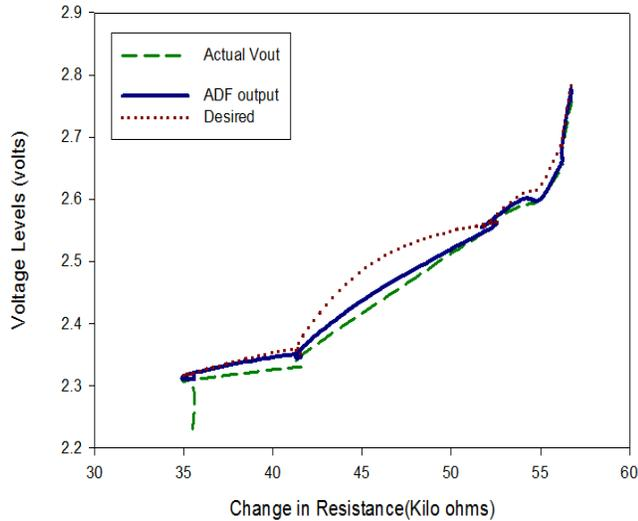
Figure 9: Comparative analysis of voltage levels in terms of bending (resistance)
