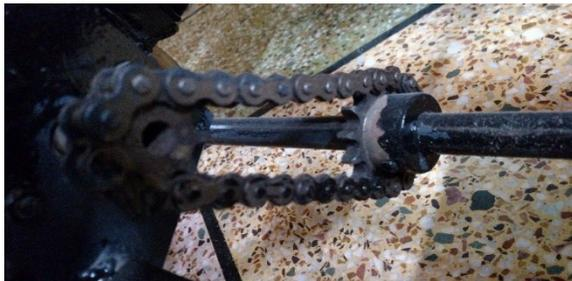
Figure 5: Chain drive and Sprocket Gear
