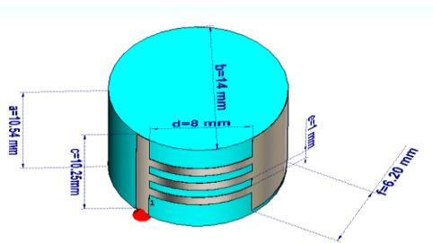
Figure 1: Configuration of the conformal Strip
