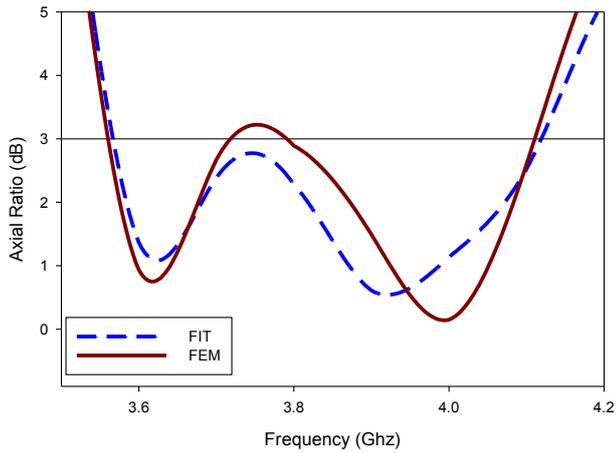
Figure 7: Validation of Axial ratio of Slotted CDRA array
