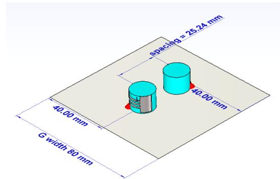
Figure 4: Geometry of Back to Back CDRA array
