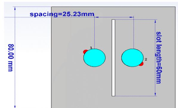
Figure 5: Top view of CDRA array with Slot.
