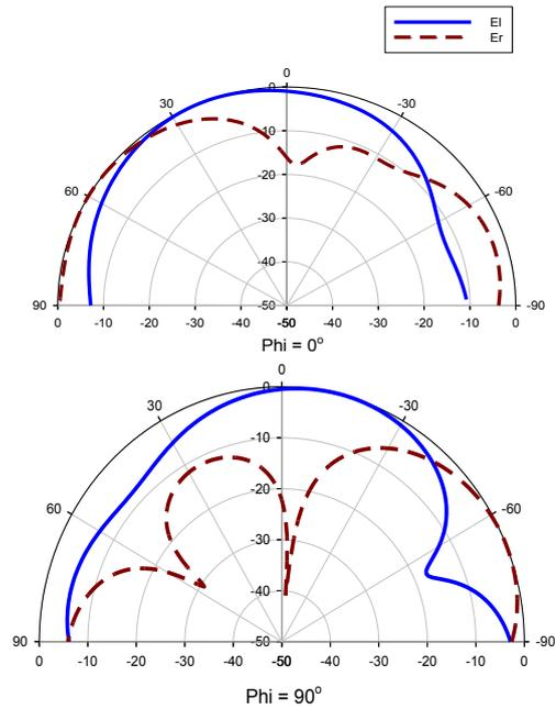
Figure 14: Radiation pattern of Slotted CDRA Array
