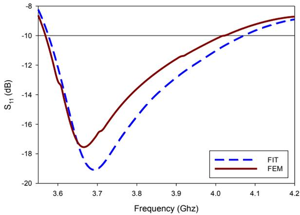
Figure 6: Validation of return loss of Slotted CDRA array
