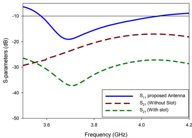
Figure 8: Reduction of MC between Slotted and without Slotted CDRA array
