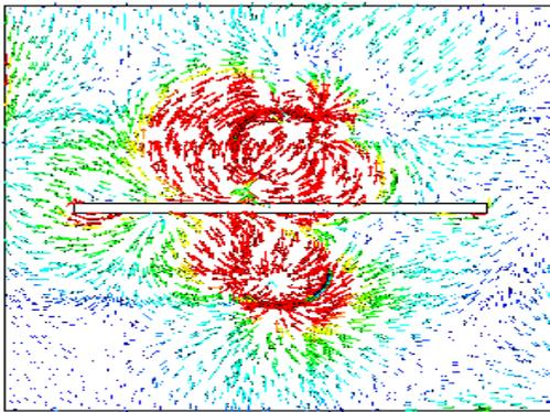
Figure 11: Change in current flow after introducing slot
