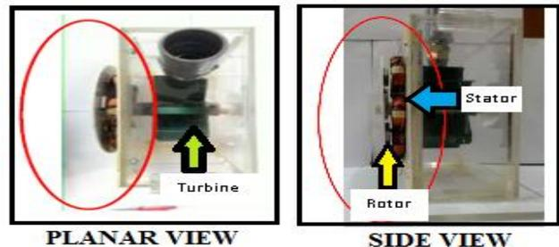
Fig. 7. Construction of generator
