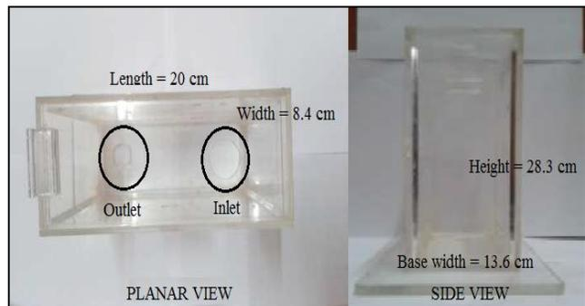
Fig. 3: Casing design of micro hydro generator
