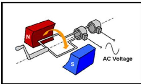
Fig. 1. Electrical generator concept [3]
