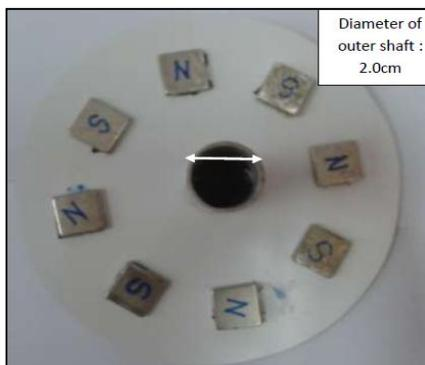
Fig. 6. Magnet arrangement
