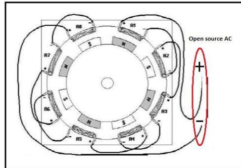
Fig. 9. Construction of stator and rotor
