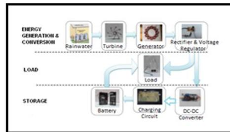
Fig. 2. Micro hydro generator system block diagram
