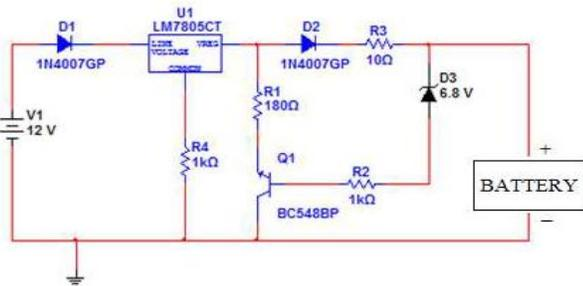
Fig.8. Charging circuit in simulation drawing
