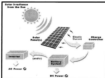
Fig. 1. Shows Solar System Block Diagram
