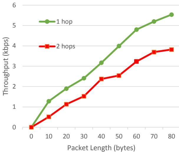
Fig 10. Throughput measurements for mulihop networks
