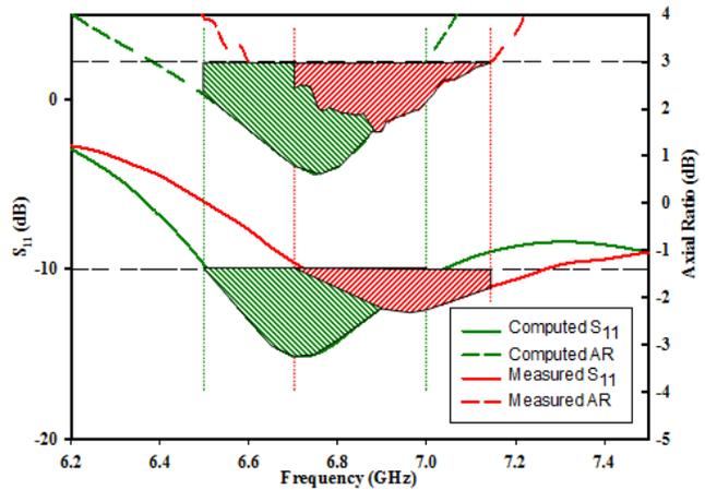
Fig. 7: Regions of overlapping bandwidths for return loss and axial ratio of the cylindrical DRA
