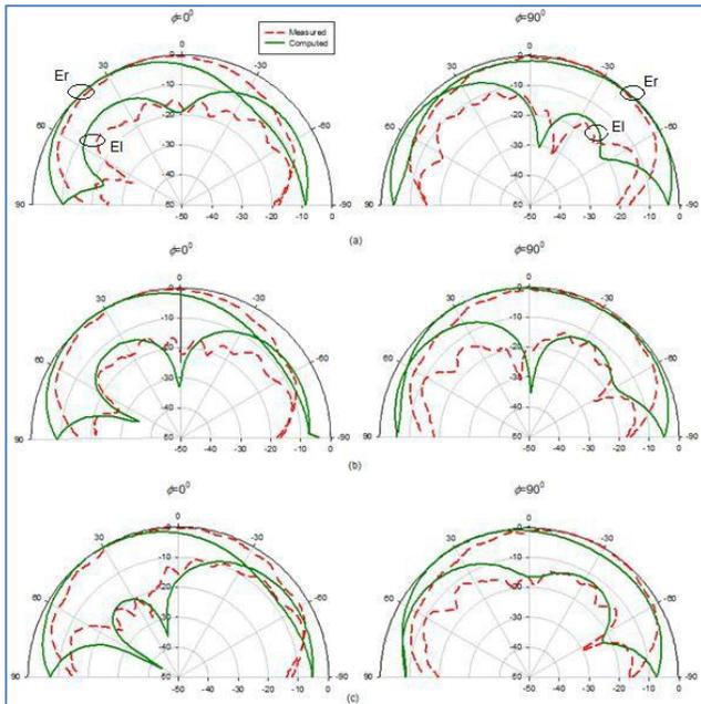
Fig. 10: Radiation patterns of the multilayer cylindrical DRA at (a) beginning, (b) centre, and (c) end of the CP bandwidth.
