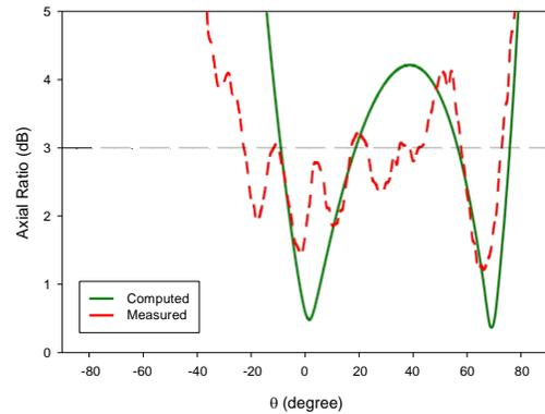
Fig. 8: AR beam-width of the cylindrical DRA at  $\phi = 0^\circ$
