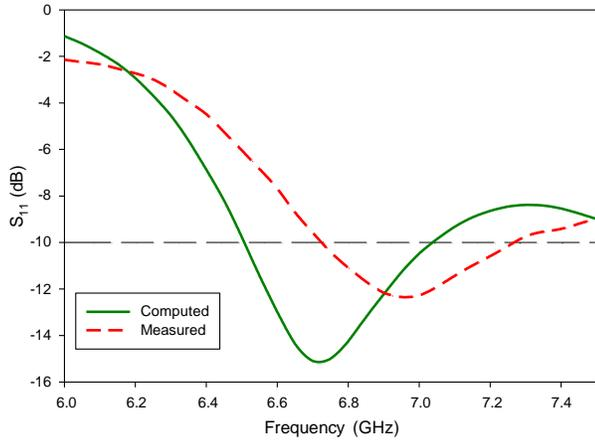
Fig. 4: Return losses of the cylindrical DRA
