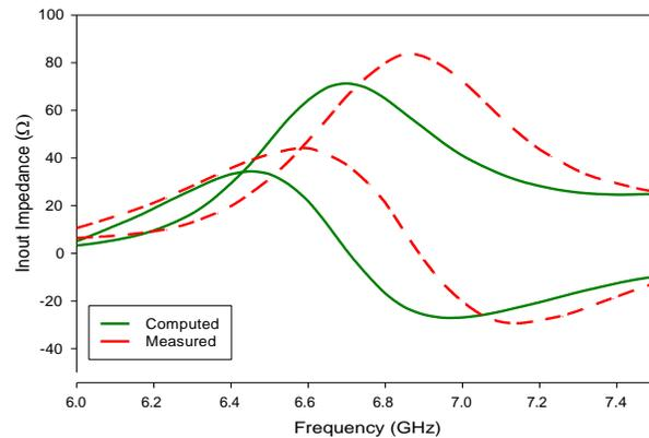
Fig. 3: Input impedance of the cylindrical DRA
