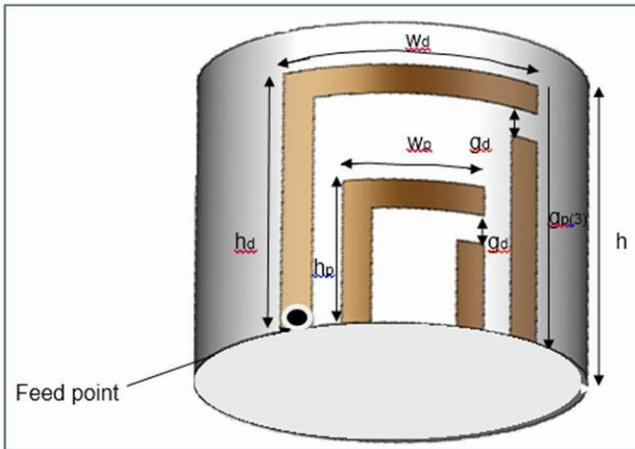
Fig. 1: Configuration of a cylindrical DRA excited by concentric open half loop
