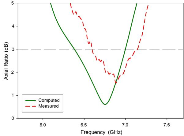
Fig. 6: Axial ratio of the cylindrical DRA
