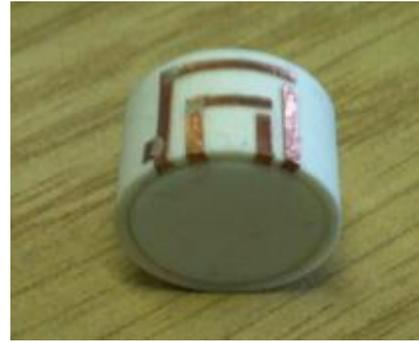
Fig. 2: Prototype of the cylindrical DRA
