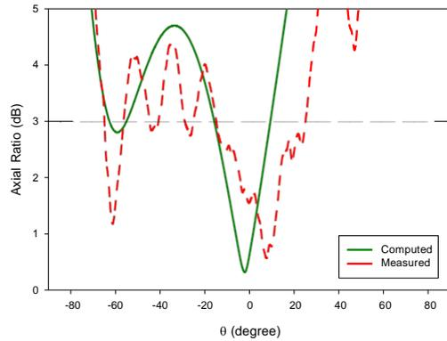
Fig. 9: AR beam-width of the cylindrical DRA at  $\phi = 90^\circ$
