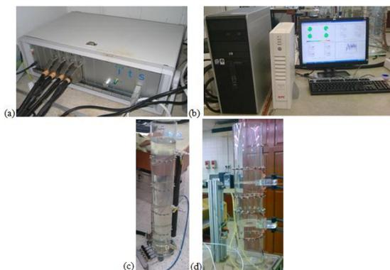
Fig. 1 Experimental apparatus: (a) data acquisition system (b) image reconstruction (c) Bubble column (d) Oscillatory Baffled Column
