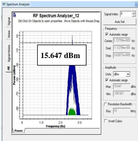
Fig. 11 Measured total post-filter in 50 km
