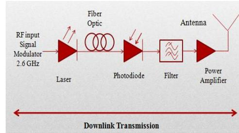
Fig. 3 Block diagram of downlink transmission
