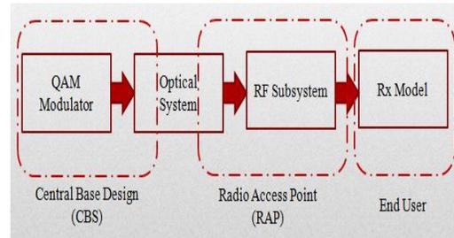
Fig. 4 Downlink Radio over Fiber Architecture
