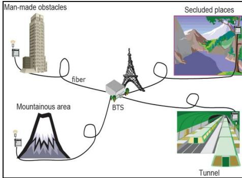
Fig. 1 Optical link for dead zone
