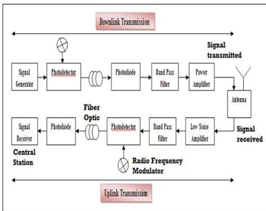
Fig. 2 Radio Access Point Architecture
