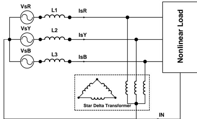
Fig. 1 Star delta transformer as a zero passing
