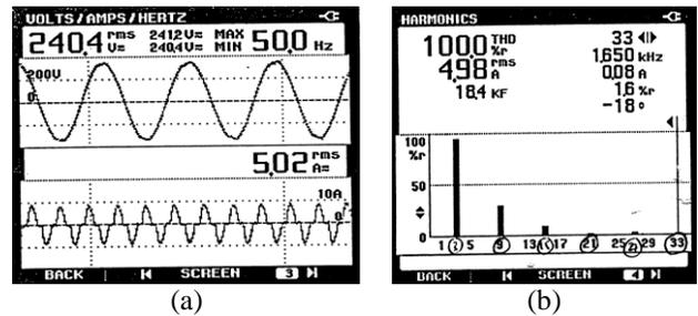
Fig. 5 Waveforms and harmonic currents before filter at Neutral line (a) Neutral current waveforms (b) Neutral harmonic currents spectrum
