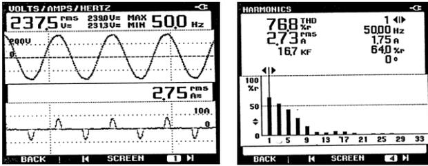
Fig. 6 Waveforms and harmonic currents after filtered by star delta transformer at line (a) Phase current waveforms (b) Harmonic currents spectrum
