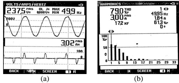
Fig. 4 Waveforms and harmonic currents before filter at line (a) Phase current waveforms (b) Harmonic currents spectrum
