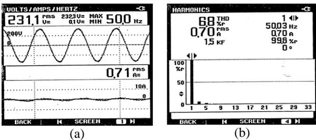
Fig. 8 Waveforms and harmonic currents after filtered by star delta transformer and LC filter at line (a) Line current waveforms (b) Line harmonic currents spectrum
