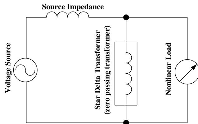
Fig. 2 The equivalent circuits for star delta transformer as a zero passing transformer
