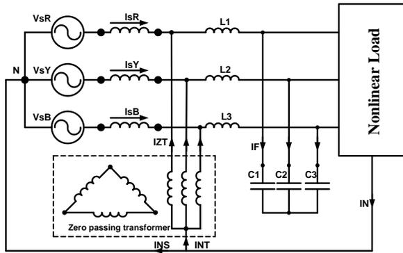
Fig. 3 The integration circuit between zero passing transformer and LC filter
