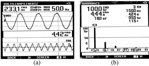
Fig.7 Waveforms and harmonic currents after filtered by star delta transformer at Neutral line (a) Neutral current waveforms (b) Neutral Harmonic currents spectrum
