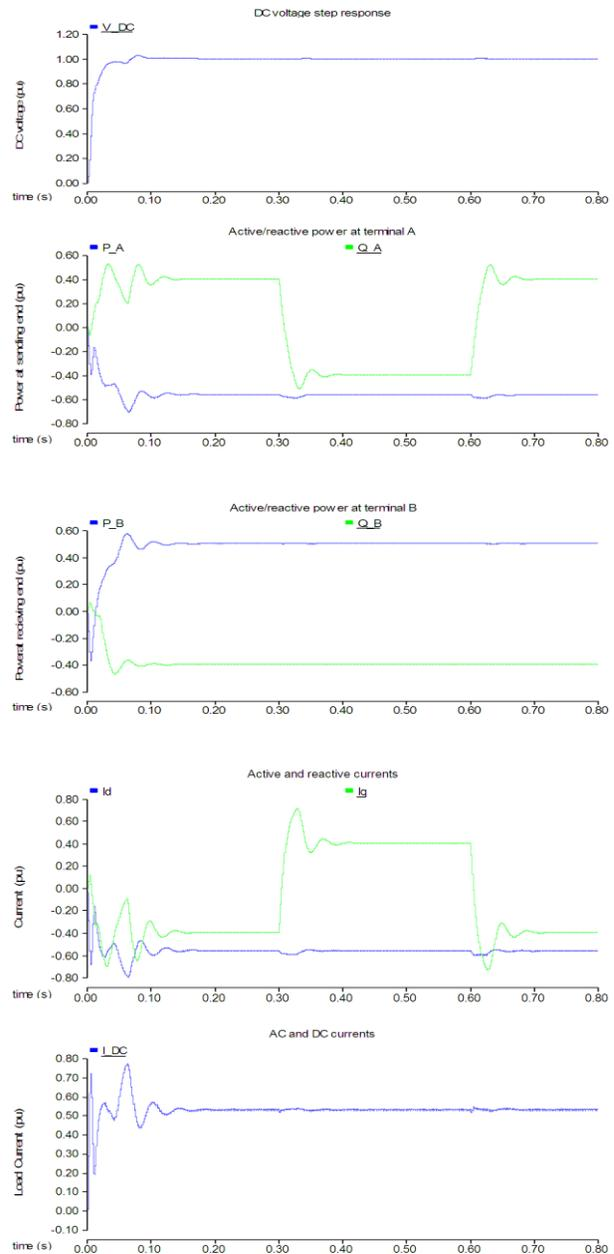
Fig. 5 Transient response for change in direction of reactive power at VSC-1.
