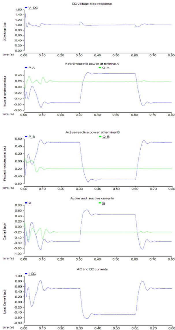
Fig. 6 Transient response for change in direction of active power at VSC-2
