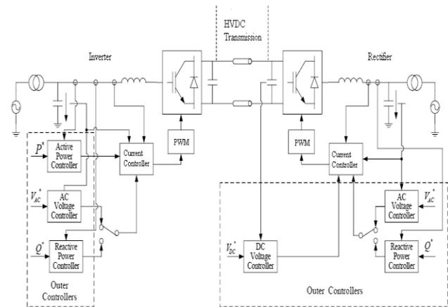
Fig 3 Overall control system of the VSC-based HVDC
