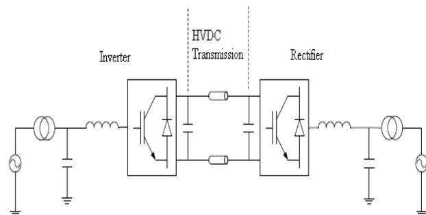
Fig 1 Configuration of a VSC-HVDC System
