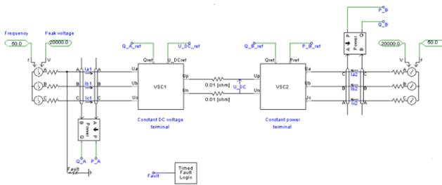
Fig. 2 Diagram of VSC-HVDC system
