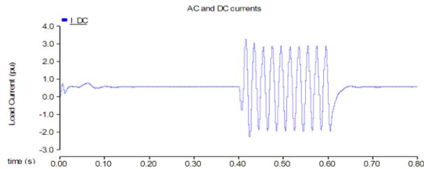
Fig. 7 Transient response for single phase to ground fault at VSC-1
