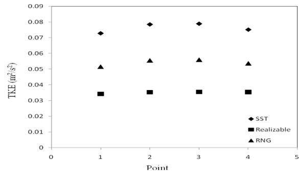
Fig. 11 Average turbulent kinetic energy with points for  $\Delta t = 0.001$  s
