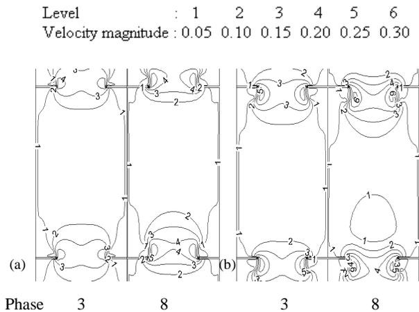
Fig. 3 Velocity vector map for SST  $k-\omega$  model at different time step size (a) 0.01 (b) 0.001.
