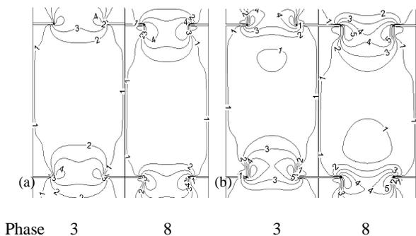
Fig. 4 Velocity vector map for Realizable  $k-\epsilon$  model at different time step size (a) 0.01 (b) 0.001.
