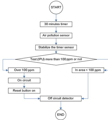
Fig. 2 Flow chart of the timer circuit
