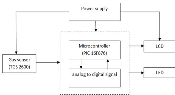
Fig. 1 Block diagram for the developed device
