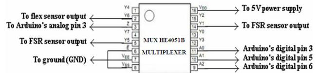
Fig. 5 HE4041BP multiplexer connection details.
