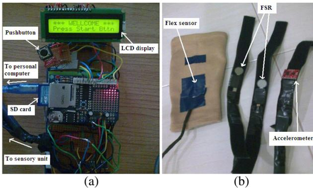
Fig. 17 Complete arm rehabilitation device consists of (a) main unit (b) sensory unit.
