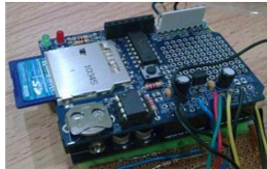
Fig. 6 Arduino data logger shields with 2 gigabytes SD card.
