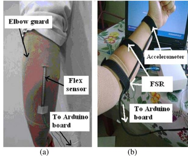
Fig. 1 (a) Elbow guard attached with flex sensor, (b) Location of the other sensors.
