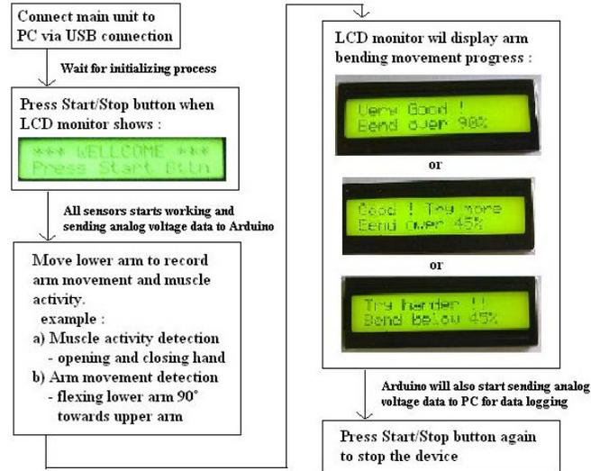
Fig. 18 Flow chart for the operation of portable arm rehabilitation device.
