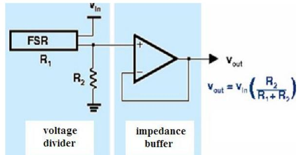
Fig. 2 Voltage divider circuitry for FSR or flex sensor.
