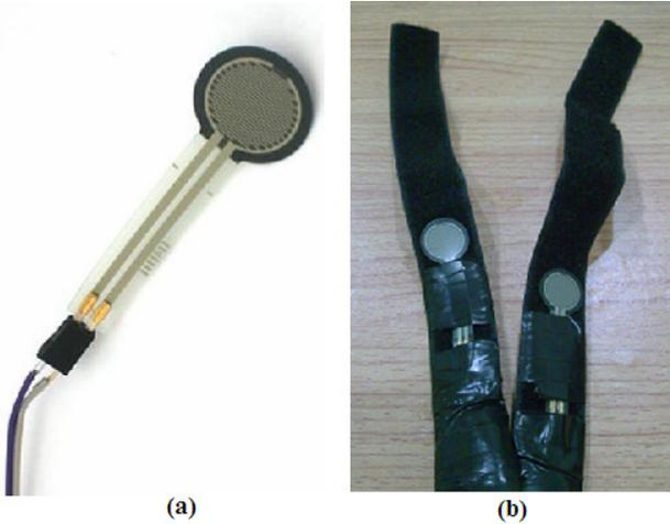
Fig. 3 (a) FSR sensor, (b) actual FSR sensors fixed on Velcro straps.
