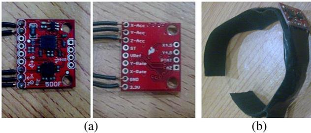
Fig. 4 (a) Left picture shows front side of IMU, while right picture shows the back side, (b) IMU attached on the Velcro strap.
