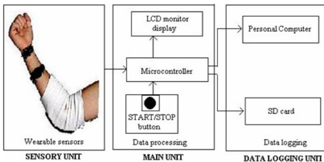
Fig. 7 Overall hardware setup diagram
