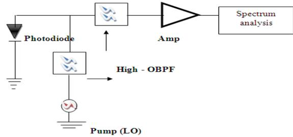
Fig. 1 Block diagram of PPA at the receiver
