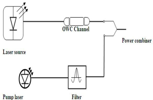
Fig. 2 Block diagram of PPA at the transmitter
