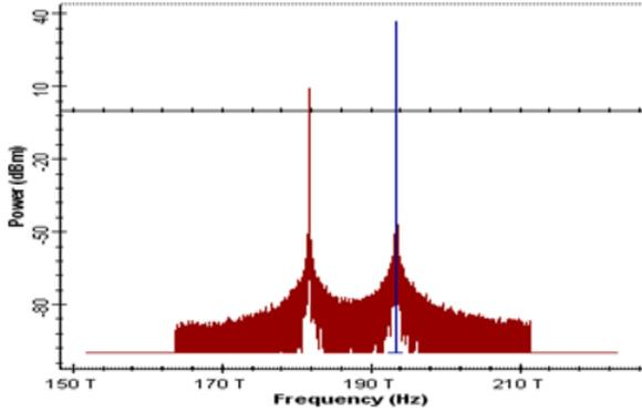
Fig. 7 Signal after the combiner (up converter)
