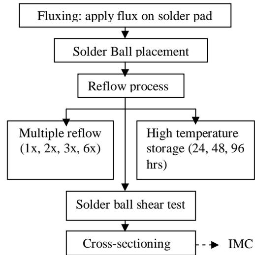
Fig 2 Experimental flow diagram
