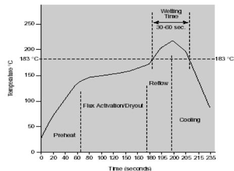
Fig. 1 Typical Reflow profile parameter for Sn/Pb
