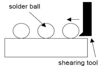
Fig. 5 Shear test diagram
