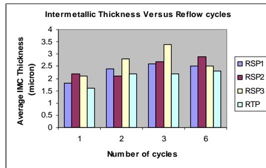
Fig. 8 IMC thickness versus reflow cycles graph
