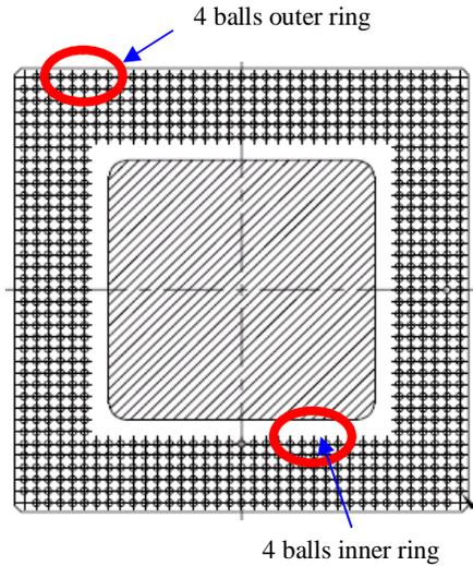
Fig. 6 TBGA unit schematic diagram
