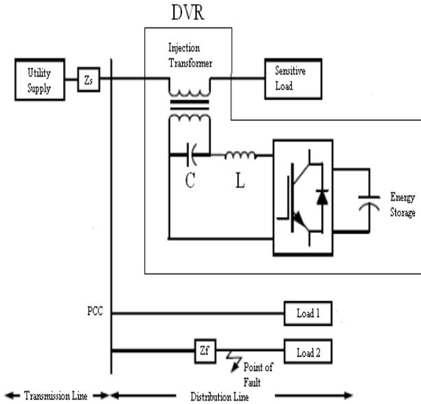
Fig. 1 Location of the Dynamic Voltage Restorer
