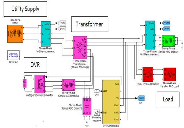
Fig. 3 Configuration of the overall of DVR in Matlab-Simpowersystem
