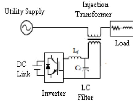
Fig. 2 Basic Components of a Dynamic Voltage Restorer
