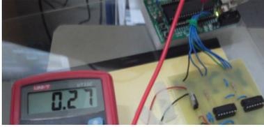
Fig. 16 Measurement on LSB input pin microcontroller
