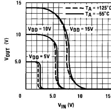
Fig. 10 Typical Performance Characteristics CD4069 [8]
