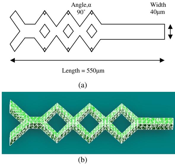
Fig. 1 The diagrams shows the dimensions of the (a) 2D model and (b) 3D solid model used in the computer simulation of mixing.
