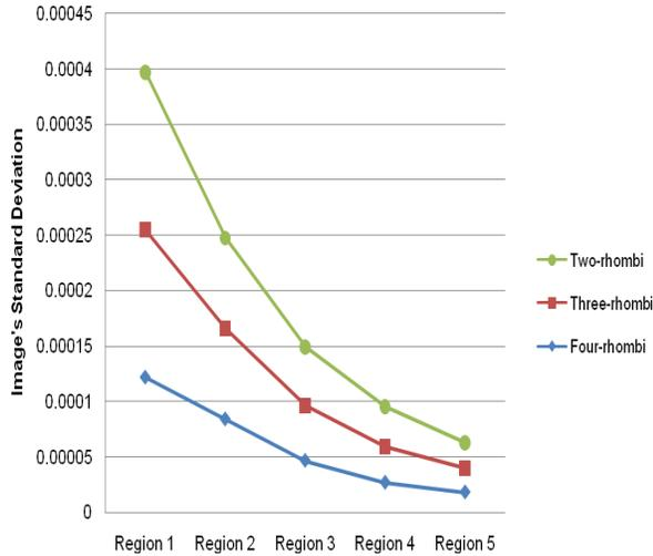
Fig. 3 Graph of image's standard deviation for laminar mixing of blood and Toluene for micromixer which consists of two, three and four rhombi.
